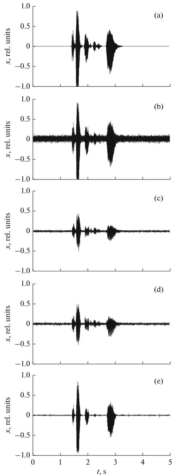
**Fig. 5.** Results of wavelet filtering of a fragment of voice message: (a) original signal, (b) signal with admixed additive noise, (c) signal after filtering by the DWT method with function (3), (d) signal after filtering by the DWT method with function (2), and (e) signal after filtering by the DCWT method.
