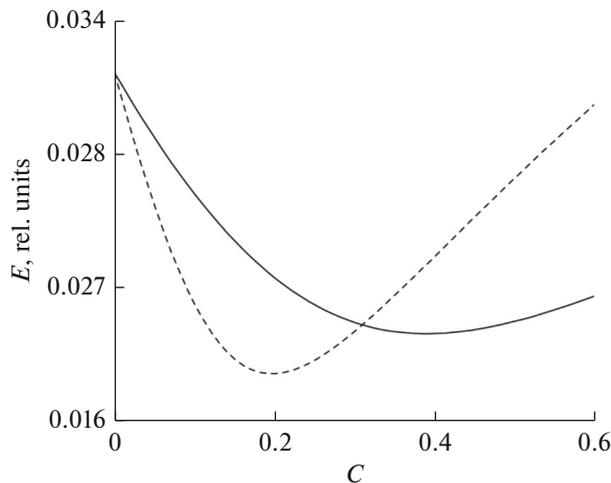
**Fig. 6.** Dependences of rms reconstruction error  $E$  on parameter  $C$  for reconstruction of the audio signal by the (solid curve) DWT and (dashed curve) DCWT methods. Calculations were performed for the Daubechies wavelet D8 (which ensured the minimum filtering error) and a noise level of 30 dB.
