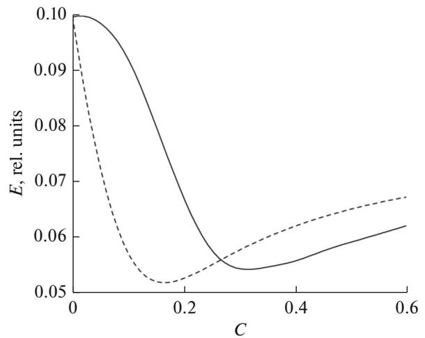
**Fig. 1.** Dependences of the rms reconstruction error on parameter  $C$  for the test signal (harmonic oscillations). The reconstruction method is based on the DWT with (solid curve) hard and (dashed curve) soft threshold functions. Calculations were performed for the Daubechies wavelet D8 and a noise level of 20 dB.
