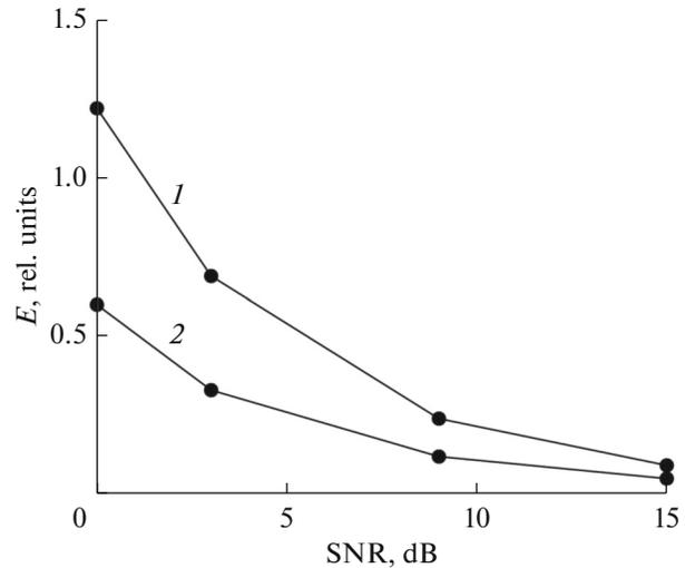
**Fig. 3.** Dependences of the optimum threshold level on the signal-to-noise ratio for the case of wavelet filtering of the test signal (harmonic oscillations) with the use of the (1) DWT and (2) DCWT methods.
