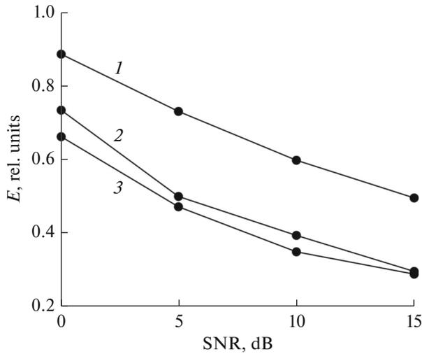
**Fig. 2.** Dependences of the rms reconstruction error on the signal-to-noise ratio for the test signal (harmonic oscillations) in the case of reconstruction based on the DWT method using the threshold function (formula (3)) and Daubechies wavelets D20: (1) the universal threshold level, (2) combined application of the universal threshold level and the SURE method, and (3) the SURE method.
