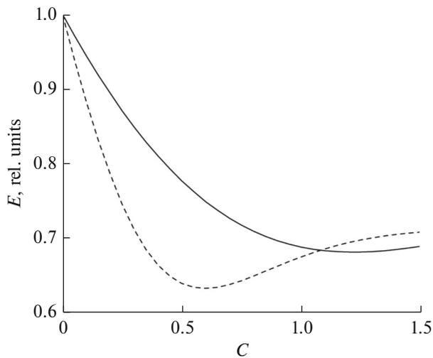
**Fig. 4.** Dependences of rms reconstruction error  $E$  on the threshold level for the case of reconstruction of the test signal (harmonic oscillations) with the use of the (solid curve) DWT and (dashed curve) DCWT methods. Calculations were performed for the Daubechies wavelet D20 and a noise level of 0 dB.
