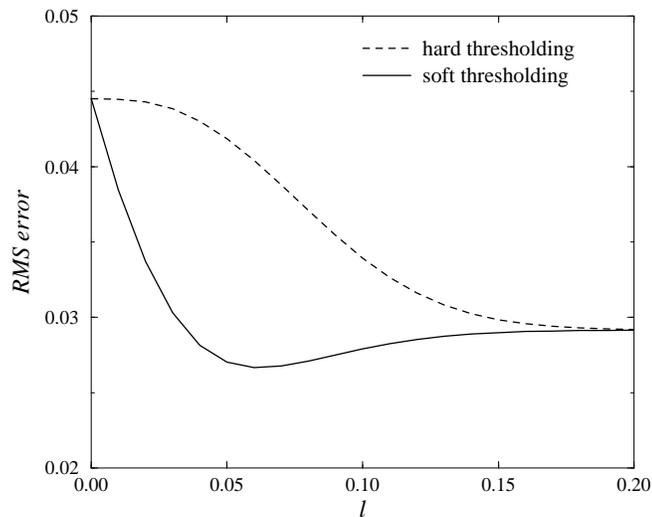
Figure 6. The dependence of RMS error vs. the threshold level for Daubechies wavelet  $D^{10}$  for hard and soft thresholding with optimal  $l = 0.2$  and  $l = 0.06$ , respectively.
