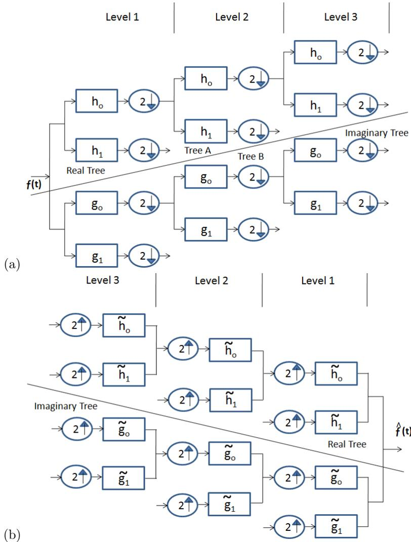
Figure 2. Analysis (a) and synthesis (b) FBs for 1-D DT-CWT.
