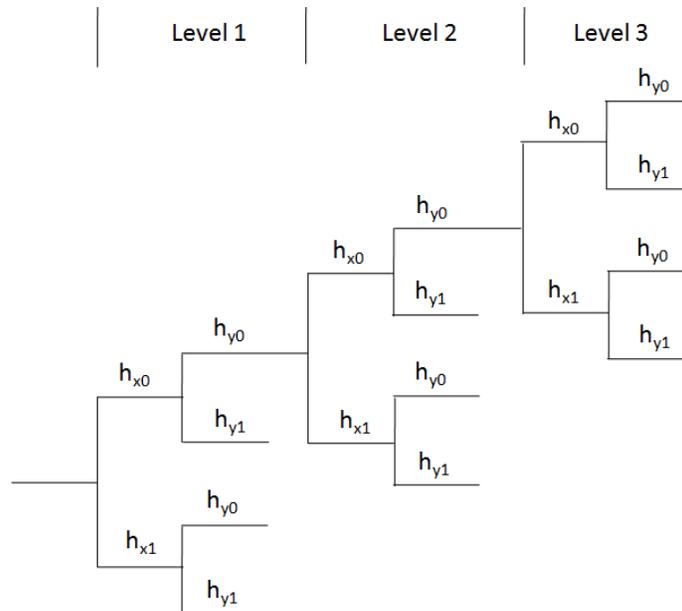
Figure 4. Filterbank structure of tree A (see Fig. 3).
