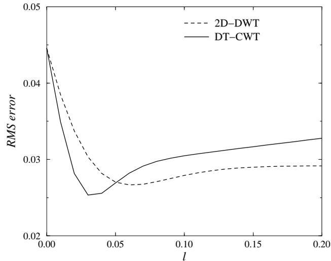
Figure 7. The dependence of RMS error vs. the threshold level for 2-D DWT and DT-CWT.
