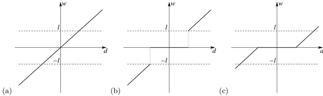
Figure 1. Threshold function associated with (a) unfiltered data, (b) hard threshold approach, and (c) soft threshold approach.
