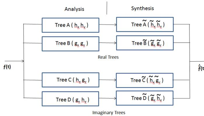
Figure 3. Filterbank structure of 2-D DT-CWT.
