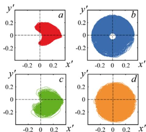
Fig. 4 Phase trajectories of the response Pierce diode on the rotating plane  $(x', y')$ : (a)  $\varepsilon = 0.058, D = 10^{-5}$  - the phase synchronization regime, (b)  $\varepsilon = 0.006, D = 10^{-5}$  - eyelet intermittency, (c)  $\varepsilon = 0.058, D = 0.03$  - ring intermittency, (d)  $\varepsilon = 0.006, D = 0.03$  - intermittency of eyelet and ring intermittencies
