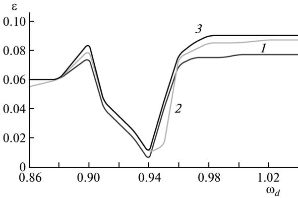
**Fig. 1.** Thresholds of the GS regime:  $a = 0.08$  (1),  $0.09$  (2), and  $0.094$  (3) for two unidirectionally coupled Rössler oscillators (2) on the plane of parameters  $(\omega_d, \varepsilon)$ .
