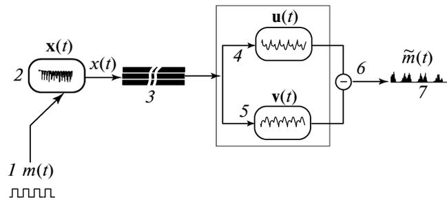
**Fig. 3.** Circuit diagram of concealed information transfer based on GS in the case of action of a chaotic signal on periodic oscillators: 1—useful binary signal  $m(t)$ ; 2—first (transmitting) oscillator; 3—communication channel; 4—second (receiving) oscillator; 5—third oscillator identical to second oscillator 4 as regards the control parameters; 6—subtractor; and 7—reconstructed useful signal  $\tilde{m}(t)$ .
