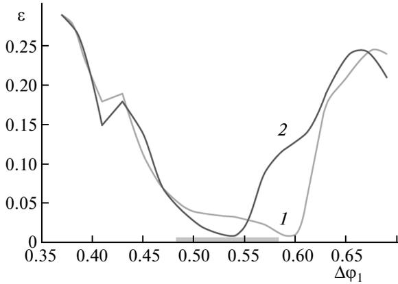
**Fig. 2.** GS thresholds in a system of two unidirectionally coupled low-voltage vircators on the plane of parameters  $(\Delta\phi_1, \varepsilon)$  for  $\Delta\phi_2 = 0.6$  (complex-periodic regime, curve 1) and  $\Delta\phi_2 = 0.525$  (chaotic regime, curve 2).
