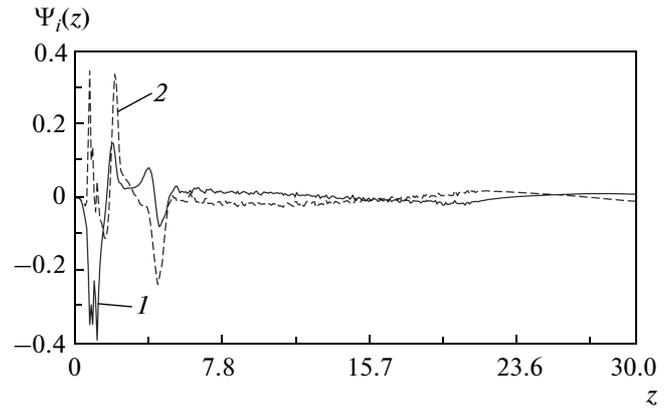
**Fig. 3.** Spatial distribution of eigenvectors  $\tilde{\Psi}_i(z)$  for the first (1) and second (2) KL modes.
