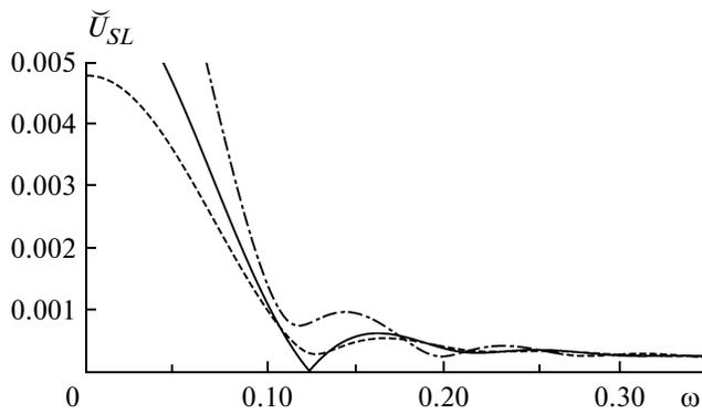
**Fig. 1.** Dependence  $\tilde{U}_{SL}(\omega)$  for when the voltage on the superlattice is less than the critical value (dashed line,  $U_{SL} = 1.14$ ), corresponds to the critical value (solid line,  $U_{SL}^* = 1.25$ ), and lies above the critical value (dash-dotted line,  $U_{SL} = 1.55$ ).
