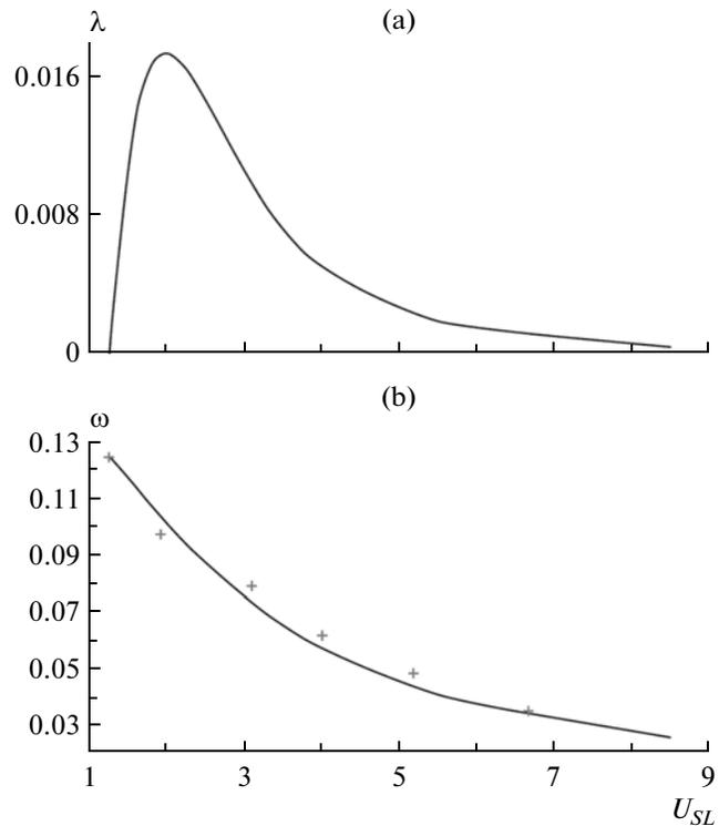
**Fig. 2.** Dependences of (a) the increment of growth and (b) the oscillation frequency of a perturbation on the applied voltage. The dots in (b) show the frequency of oscillations for a current flowing through a superlattice, calculated numerically.
