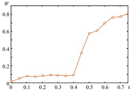
**Fig. 6.** Dependence of chaotic signal bandwidth  $W$  averaged over all oscillators of the network on the coupling parameter value  $\varepsilon$ .
