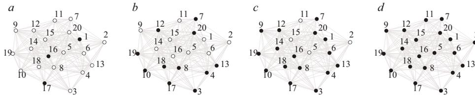
**Fig. 5.** The evolution of the synchronous cluster in the random network of  $N = 20$  elements on the frequency  $f = 2.67$  GHz with the coupling parameter value increasing: (a)  $\varepsilon = 0.15$ ; (b)  $\varepsilon = 0.225$ ; (c)  $\varepsilon = 0.275$ ; (d)  $\varepsilon = 0.375$ . The asynchronous generators are shown by white circles, the generators being in the time scale synchronization regime are marked by black.
