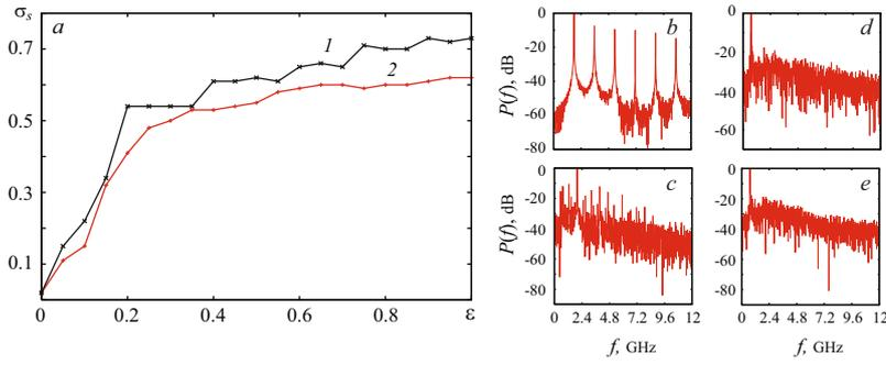
**Fig. 3.** (a) Dependencies of the synchronization index  $\sigma_s$  on the coupling parameter  $\epsilon$  for the simply ordered chain of  $N = 10$  low-voltage vircators with slightly (curve 1) and strongly (curve 2) detuned control parameter values. (b-e) Power spectra of output signals of first (b,d) and seventh (c,e) low-voltage vircators for the different values of the coupling parameter, i.e.  $\epsilon = 0$  (b,c),  $\epsilon = 0.2$  (d,e).
