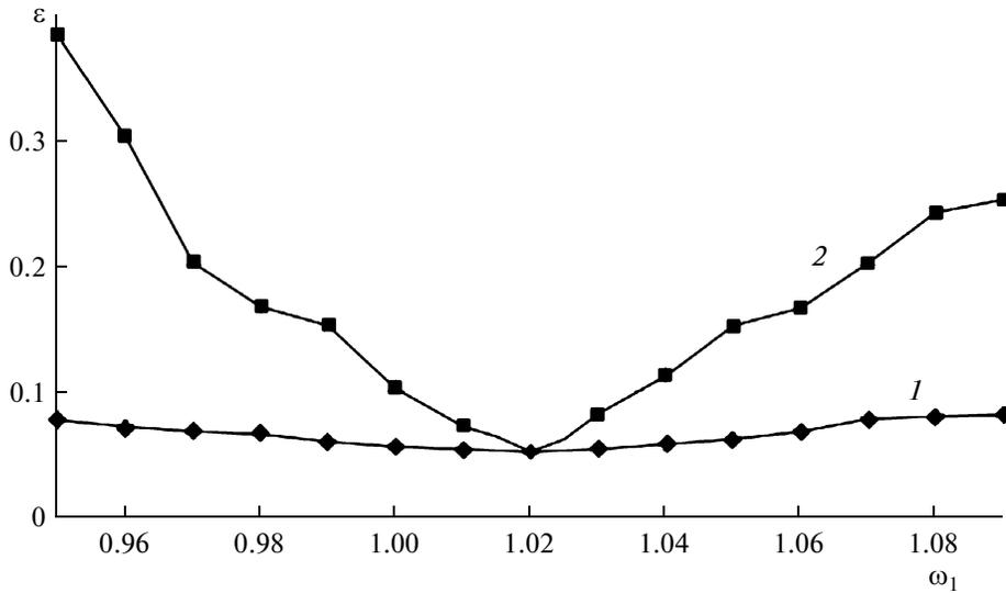
**Fig. 4.** Boundaries of the (1) generalized synchronization and (2) time-delay synchronization regimes in system (8) of two mutually coupled tunnel-diode oscillators.
