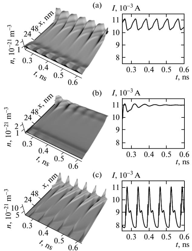
**Fig. 4.** Space–time diagrams characterizing the evolution of charge domains as a function of time and coordinate, and current  $I(t)$  through the superlattice at temperature of  $T = 200$  K and voltage of (a)  $V = 0.54$  V, (b)  $V = 0.55$  V, and (c)  $V = 0.56$  V.
