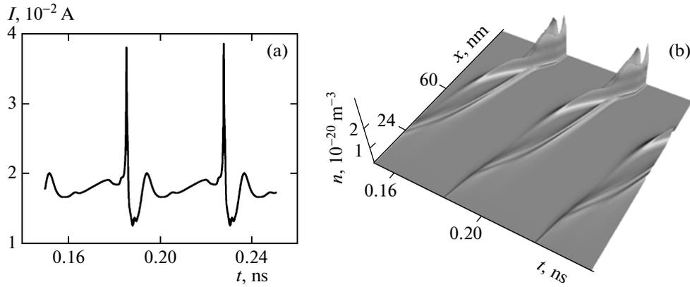
**Fig. 2.** (a) Current  $I(t)$  through a superlattice for  $T = 0$  and  $V = 0.61$  V. (b) Space–time diagram characterizing the evolution of charge domains as a function of time and coordinate.
