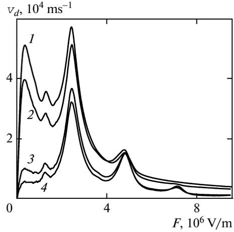
**Fig. 1.** Drift velocity of an electron as a function of electric field strength for various temperatures and a magnetic field of  $B = 15$  T with a tilt angle of  $\theta = 40^\circ$ . Curve 1 corresponds to the temperature of  $T = 0$  K, curve 2, to  $T = 50$  K, curve 3, to  $T = 200$  K, and curve 4, to  $T = 300$  K.
