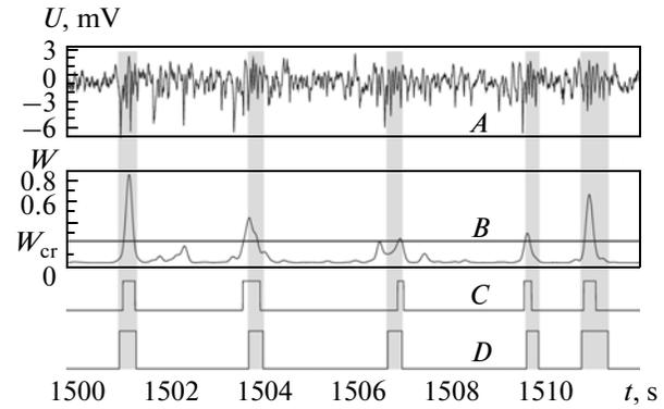
**Fig. 3.** (A) EEG segment, (B) average energy  $|W(t, f)|$  of WCT in the frequency range of 9–16 Hz, and (C) the results from automatic marking, i.e., the marking of sleep spindles, along with (D) a comparison with expert markings. The time of the occurrence of sleep spindles in the EEG signal is shown in gray.
