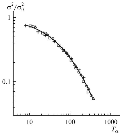
**Fig. 2.** Dependence of the dispersion of the phase difference distributions of unidirectionally coupled Pierce diodes on the normalized length of the investigated time series  $T_\alpha$  for the value of the coupling parameter:  $\epsilon = 0.008$  (crosses),  $\epsilon = 0.01$  (squares),  $\epsilon = 0.012$  (circles),  $\epsilon = 0.014$  (triangles).
