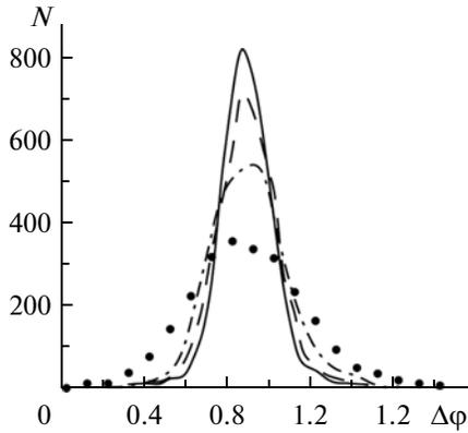
**Fig. 1.** Distributions of the phase difference of two unidirectionally Pierce diodes at  $\varepsilon = 0.01$ :  $T = 3900$  (solid line);  $T = 3000$  (dotted line);  $T = 1950$  (dashed-and-dotted line);  $T = 750$  (points).
