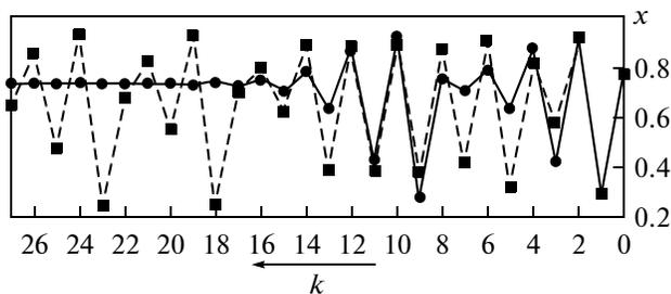
**Fig. 1.** Dependence of coordinate  $x$  of logistic map (14) on the discrete length of prehistory  $k$ . Reference trajectory  $x_{N-k}$  is shown with a solid line; the trajectories  $x_{J1-k}$  and  $x_{J2-k}$  (whose final points  $x_{J1}$  and  $x_{J2}$  are close to  $x_N$ ) are shown by dots  $\bullet$  (line 1) and the dashed line with dots  $\blacksquare$  (line 2), respectively.
