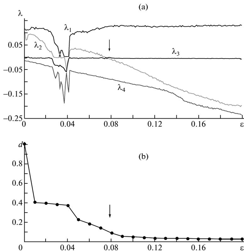
**Fig. 1.** Plots of (a) four highest Lyapunov exponents  $\lambda$  and (b) quantitative measure of proximity  $d$  versus coupling parameter  $\varepsilon$ . The arrow indicates the critical value  $\varepsilon_c = 0.078$  of the coupling parameter that corresponds to the appearance of GS in the system of mutually coupled BPSs.
