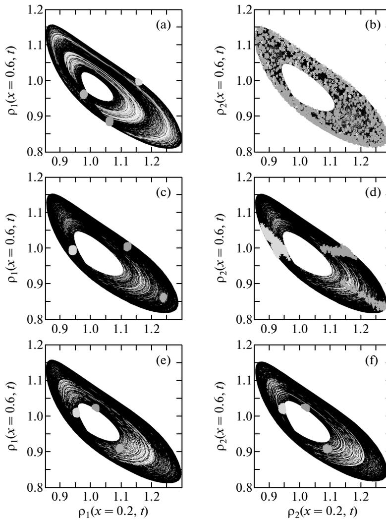
**Fig. 2.** Reconstructed attractors of mutually coupled Pierce diodes plotted on the plane  $[\rho_{1,2}(x = 0.2, t), \rho_{1,2}(x = 0.6, t)]$  for various values of coupling coefficient  $\varepsilon$ : (a, b) 0.002 (asynchronous state); (c, d) 0.05 (phase synchronization); (e, f) 0.10 (GS regime); (a, c, e) reconstructed attractors of first Pierce diode with randomly chosen points; (b, d, f) phase space of second system with the corresponding nearest-neighbor states.
