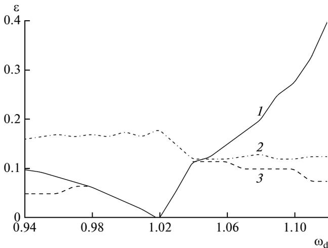
**Fig. 1.** Boundaries of the appearance of (1) PS, (2) GS, and (3) phase-coherent attractor plotted on the plane of control parameters ( $\omega_d$ ,  $\varepsilon$ ) for system (1) of two unidirectionally coupled oscillators based on tunnel diodes.
