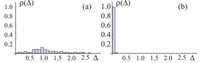
FIG. 4. Histograms of the normalized difference  $\Delta = \|\delta\mathbf{y}_i(t) - \delta\mathbf{z}_i(t)\| / \|\delta\mathbf{y}_i(t)\|$  for (a) the asynchronous dynamics ( $\varepsilon = 0.06$ ) and (b) the generalized synchronization regime ( $\varepsilon = 0.3$ ). The histograms have been obtained for the response Rössler system [Eq. (7)]. The length of the phase tube is  $\tau = 100$ .
