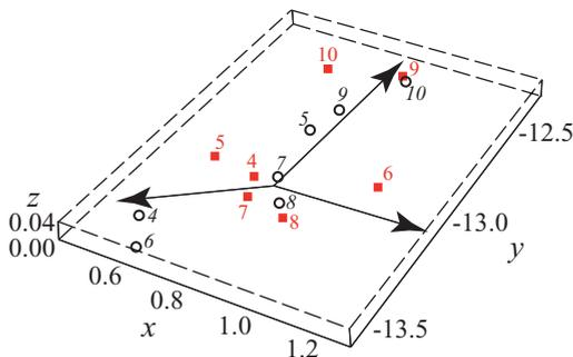
FIG. 1. (Color online) Vectors  $\mathbf{y}_i$  (■) and  $\mathbf{z}_i$  (○) of the response Rössler system [Eq. (7)] for  $\varepsilon = 0.3$ . The numbers  $i$  of the vectors are shown by the roman and italic fonts, respectively
