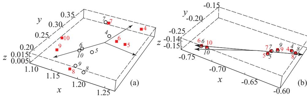
FIG. 5. (Color online) Vectors  $\mathbf{y}_i$  (■) and  $\mathbf{z}_i$  (○) of the second generator with a tunnel diode [Eq. (14)] for  $\varepsilon = 0.15$ . The numbers  $i$  of the vectors are shown by the roman and italic fonts, respectively. (a) All neighbor vectors are used. (b) Only vectors whose phase trajectories pass through the phase tube with length  $\tau = 110$  are used.
