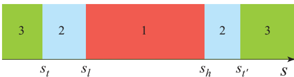
FIG. 2. (Color online) Schematic representation of the regimes observed for the different values of the observation time scale s . 1: synchronous dynamics; 2: intermittent behavior; 3: asynchronous behavior. The coupling strength between oscillators is supposed to be fixed.
