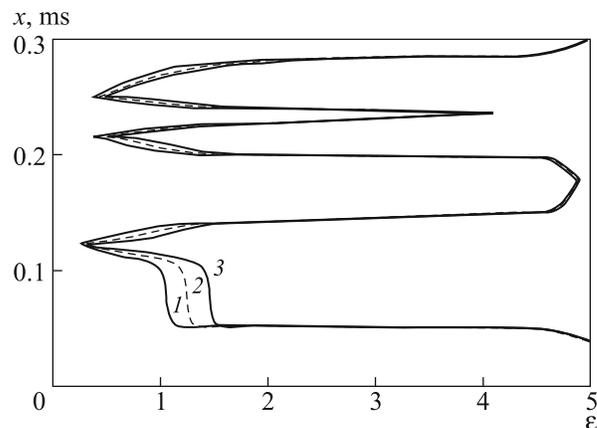
**Fig. 2.** Dependences of the synchronous scale range on the coupling parameter  $\varepsilon$ : (1) external source noise is absent and (2, 3) SNR = 5 and 1, respectively.
