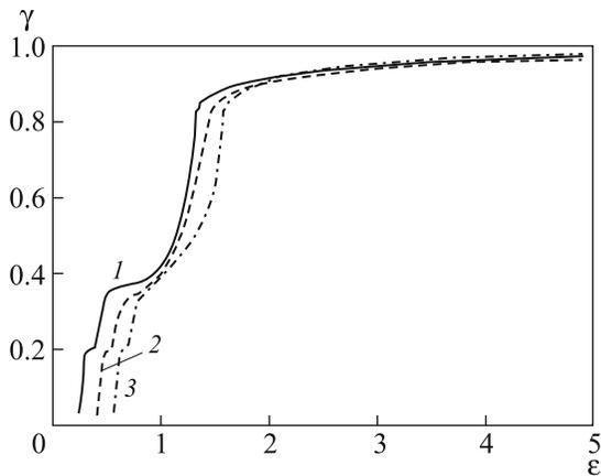
**Fig. 3.** Dependences of the synchronization measure of chaotic oscillators on the coupling parameter  $\varepsilon$ : (1) external source noise is absent and (2, 3) SNR = 5 and 1, respectively.
