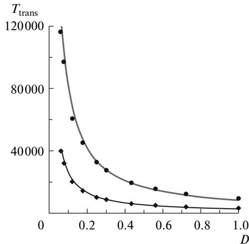
**Fig. 2.** Dependences of the mean transition time of synchronous ( $T_{\text{trans}}$ ) oscillations of Van der Pol oscillators (1) from the noise intensity ( $D$ ) at zero amplitude of the exterior signal ( $\bullet$ ) and at  $A < A_c$ ,  $A = 0.022$  ( $\blacklozenge$ ) approximated by power functions with exponents  $(-1)$  (clear and dark lines, respectively).
