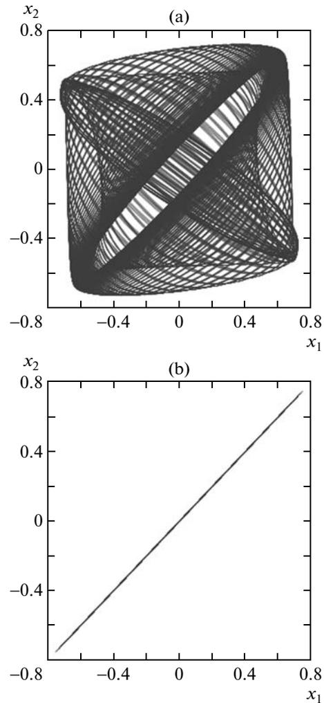
**Fig. 1.** (a) States of the first ( $x_1$ ) and second ( $x_2$ ) uncoupled nonautonomous Van der Pol oscillators (1) at certain instants at zero noise intensity ( $D = 0$ ). (b) A case of states of the first ( $x_1$ ) and second ( $x_2$ ) uncoupled nonautonomous Van der Pol oscillators (1) at certain instants at non-zero noise intensity ( $D = 0.5$ ).
