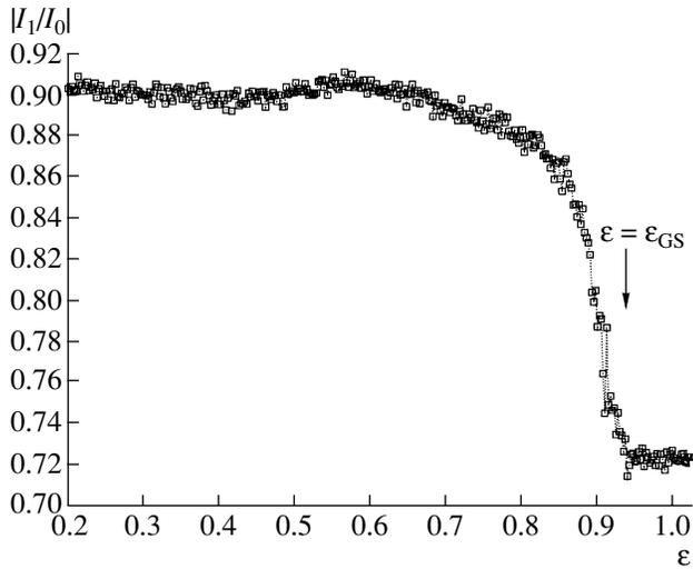
**Fig. 2.** A plot of the time-averaged relative amplitude of the first harmonic of the electron bunch current  $I_1/I_0$  in the response klystron autooscillator versus coupling parameter  $\varepsilon$ . The arrow indicates the value of  $\varepsilon = \varepsilon_{GS}$  for which the GS regime is established.
