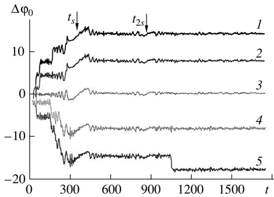
**Fig. 4.** Phase difference  $\Delta\varphi_0(t)$  at a time scale  $s_1 = s_0 + \Delta s$  approximately matching the scale  $s_0 = 1/f_0 = 10.28$  of the autonomous van der Pol oscillator,  $s_1 = (1)$   $11.46 > s_0$ ,  $(2)$   $11.24 > s_0$ ,  $(3)$   $10.28 = 2s_0$ ,  $(4)$   $8.55 < s_0$ , and  $(5)$   $8.52 < s_0$ .
