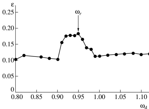
**Fig. 1.** The boundary of the region corresponding to the onset of the GS regime on the plane of control parameters  $(\omega_d, \epsilon)$  for a system of two unidirectionally coupled Rössler oscillators. The arrow indicates the  $\omega_r$  value of the response system.
