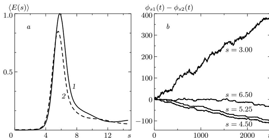
**Fig. 5.** (a) The normalized energy distribution in the wavelet spectrum  $\langle E(s) \rangle$  for the first (line 1) and the second (line 2) Rössler systems; (b) the phase difference  $\phi_{s1}(t) - \phi_{s2}(t)$  for two coupled Rössler systems. The value of coupling parameter is selected as  $\varepsilon = 0.025$ . There is no phase synchronization between the systems
