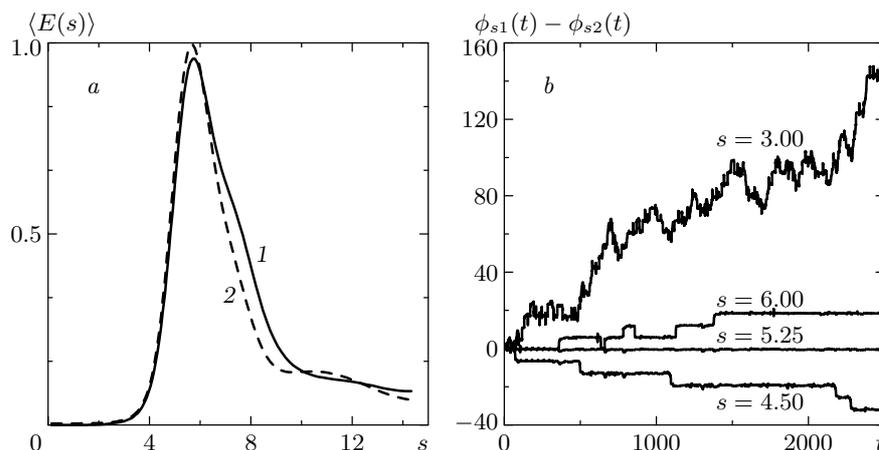
**Fig. 4.** (a) The normalized energy distribution in the wavelet spectrum  $\langle E(s) \rangle$  for the first (line 1) and the second (line 2) Rössler systems (11); (b) the phase difference  $\phi_{s1}(t) - \phi_{s2}(t)$  for two coupled Rössler systems. The value of the coupling parameter is selected as  $\varepsilon = 0.05$ . The time scales  $s = 5.25$  are correlated with each other and synchronization is observed
