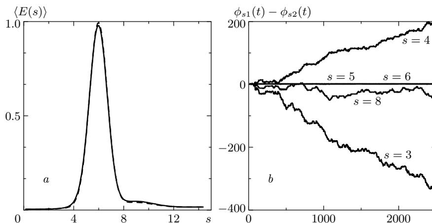
Fig. 2. (a) Wavelet power spectra  $\langle E(s) \rangle$  for the first (solid line) and the second (dashed line) Rössler systems (10). (b) The dependence of the phase difference  $\phi_{s1}(t) - \phi_{s2}(t)$  on time  $t$  for different time scales  $s$ . The coupling parameter between the oscillators is  $\varepsilon = 0.05$ . Phase synchronization for two coupled chaotic oscillators is observed
