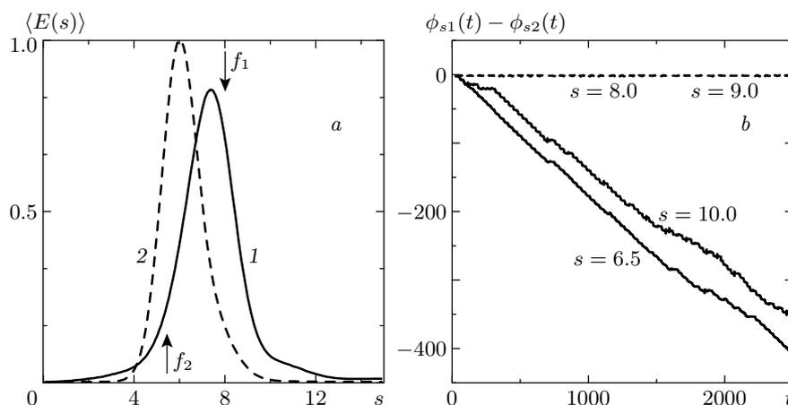
Fig. 10. (a) The normalized energy distribution in the wavelet spectrum  $\langle E(s) \rangle$  for the first (line 1) and the second (line 2) Rössler systems. The time scales indicated with arrows correspond to the frequencies  $f_1 = 0.125$  and  $f_2 = 0.154$ ; (b) the phase difference  $\phi_{s1}(t) - \phi_{s2}(t)$  for two coupled Rössler systems. The generalized synchronization is observed
