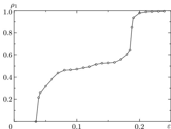
**Fig. 11.** The dependence of the synchronization measure  $\rho_1$  for the first Rössler system (11) on the coupling strength  $\varepsilon$ . The measure  $\rho_2$  for the second Rössler oscillator behaves in a similar manner (not shown in the figure)
