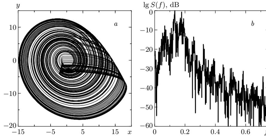
**Fig. 3.** (a) A phase picture and (b) the power spectrum of oscillations for the first Rössler system (11). The coupling parameter  $\varepsilon$  is equal to zero
