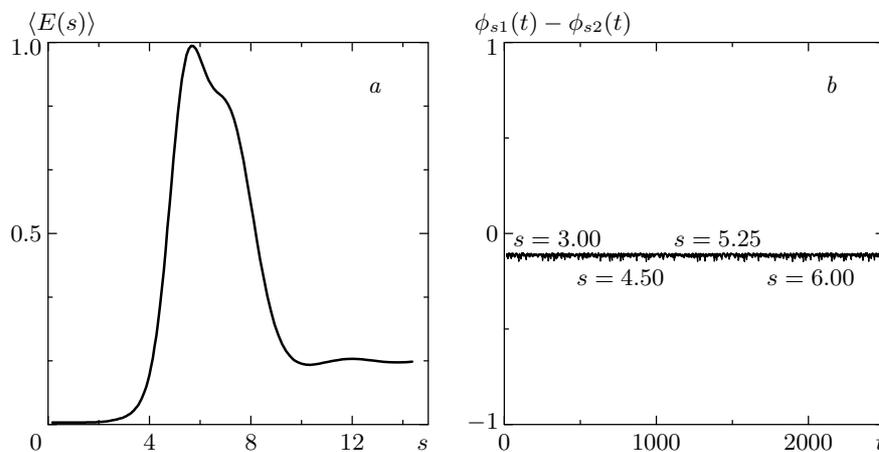
**Fig. 7.** (a) The normalized energy distribution in the wavelet spectrum  $\langle E(s) \rangle$  for the Rössler system; (b) the phase difference  $\phi_{s1}(t) - \phi_{s2}(t)$  for two coupled Rössler systems. The value of the coupling parameter is selected as  $\varepsilon = 0.25$ . Lag synchronization is observed, all time scales are synchronized
