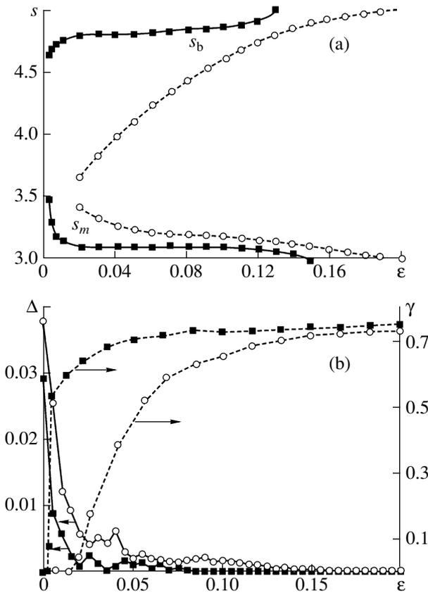
**Fig. 1.** Plots of (a) the lower ( $s_m$ ) and upper ( $s_b$ ) boundaries of the interval of synchronized time scales and (b) the parameter of identity ( $\Delta$ ) and relative energy ( $\gamma$ ) of the synchronized spatiotemporal oscillations versus coupling parameter  $\varepsilon$  for the two coupled Pierce diodes with small ( $\alpha_1/\pi = 2.860$ ,  $\alpha_2/\pi = 2.861$ ) (■) and large ( $\alpha_1/\pi = 2.860$ ,  $\alpha_2/\pi = 2.858$ ) (○) detunings.
