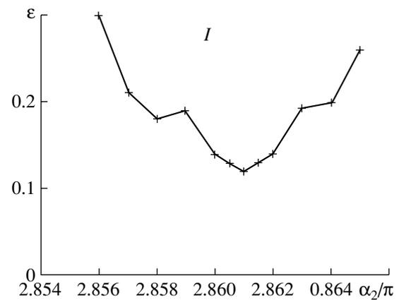
**Fig. 2.** The boundary of the region (I) of complete chaotic synchronization between two coupled distributed beam-plasma systems (Pierce diodes) on the plane of control parameters  $(\alpha_2/\pi, \varepsilon)$  for the constant value of  $\alpha_1 = 2.861\pi$ .
