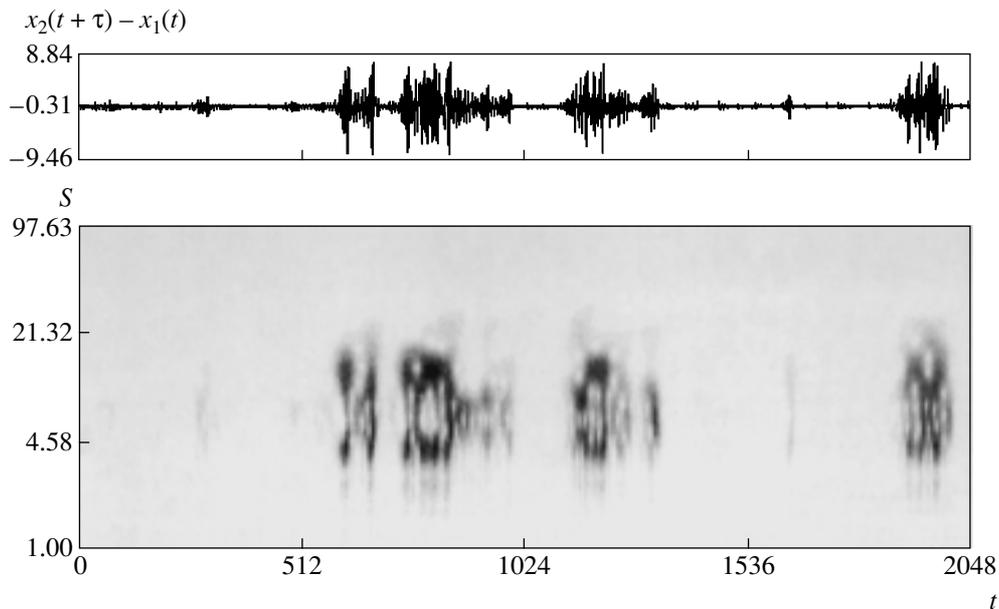
**Fig. 1.** The regime of intermittent lag synchronization between two coupled Rössler systems (2) with  $\varepsilon = 0.13$  ( $\tau = 0.32$ ): (a) the typical time series of the differential signal  $\mathbf{x}_2(t + \tau) - \mathbf{x}_1(t)$ ; (b) the corresponding projection of the wavelet surface modulus  $|W(t, s)|$ .
