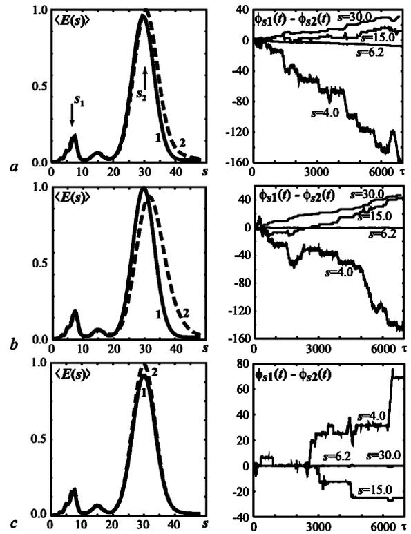
FIG. 6. Wavelet power spectra of time series  $x_{1,2}(t)$  of two coupled Chua's circuit (11) (solid line "1" corresponds to the first Chua's circuit, dashed line corresponds to the second circuit, respectively) and phase difference  $\phi_{s_1}(t) - \phi_{s_2}(t)$  on different time scales  $s$ . The value of the coupling parameter  $\varepsilon$  is (a)  $\varepsilon = 0.0$ , (b)  $\varepsilon = 0.05$ , and (c)  $\varepsilon = 0.25$ .
