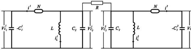
FIG. 4. Circuit realization of two mutually coupled Chua's oscillators.
