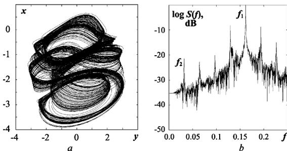
FIG. 5. The chaotic attractor and Fourier spectrum of the first Chua's circuit. The coupling parameter  $\varepsilon$  is equal to zero.
