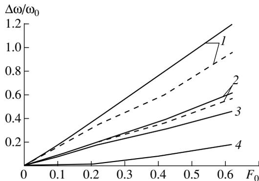
**Fig. 4.** Synchronization (dashed line) and quasi-synchronization (solid line) bandwidths vs. external signal amplitude  $F_0/F_{out}$  at  $A = (1) 2.1, (2) 2.4, (3) 2.8,$  and  $(4) 3.5$  ( $F_{out}$  is the output signal amplitude in the autonomous mode).
