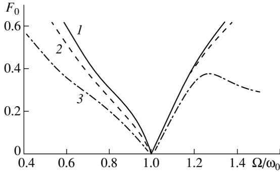
**Fig. 3.** The plane of control parameters—external signal frequency  $\Omega$  and amplitude  $F_0$ —divided into regions corresponding to characteristic nonautonomous oscillation modes realized in a BWT: (1) synchronization mode, (2) quasi-synchronization region, and (3) change in the character of self-modulation.
