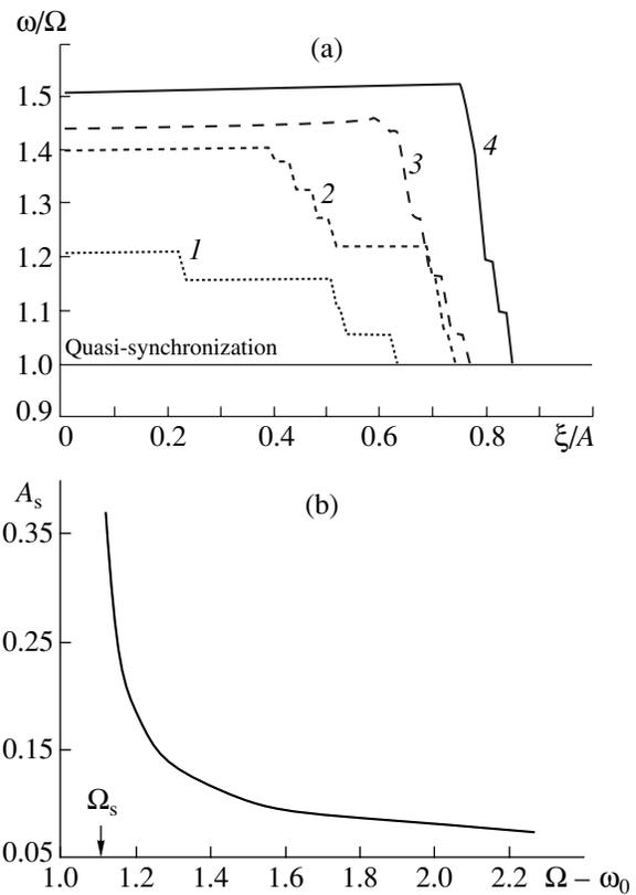
Fig. 7. (a) The characteristic self-oscillation frequency in various sections of the interaction space obtained at different external signal frequencies,  $\Omega - \omega_0 = (1)$  1.13, (2) 1.15, (3) 1.18, and (4) 1.28, and (b) synchronization length  $A_s$  vs. detuning ( $A = 2.2$  and  $F_0/F_{out} = 0.3$ ).
