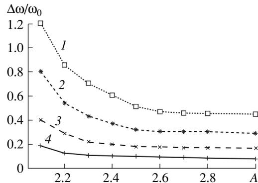
**Fig. 5.** Synchronization bandwidth  $\Delta\omega/\omega_0$  vs. system length  $A$  obtained at various control signal amplitudes  $F_0/F_{out}$  (calculations are performed using nonlinear nonstationary model (1)–(3)):  $F_0/F_{out} = (1) 0.45, (2) 0.3, (3) 0.15,$  and  $(4) 0.1$ .
