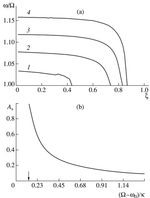
**Fig. 2.** (a) Oscillation frequency vs. interaction space coordinate  $\xi$  obtained at various detuning values:  $|\Omega - \omega_0|/\kappa =$  (1) 0.23, (2) 0.45, (3) 0.68, and (4) 0.91. (b) Synchronization length  $A_s$  vs.  $|\Omega - \omega_0|/\kappa$ .
