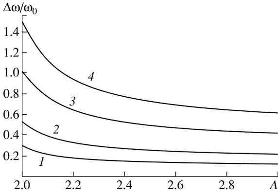
**Fig. 1.** Synchronization bandwidth  $\Delta\omega/\omega_0$  vs. control parameter  $A$  obtained at  $E_0/E_{out} = (1)$  0.1, (2) 0.15, (3) 0.3, and (4) 0.45.
