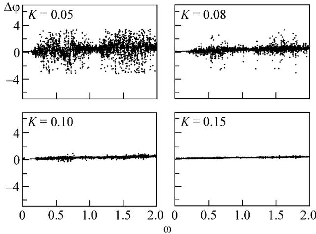
**Fig. 3.** Phase difference  $\Delta\phi$  for the different Fourier components of the coupled Ressler systems. Since the phase difference between the synchronized spectral components obeys Eq. (7), the value of  $\Delta\phi$  for the locked-in frequencies should fall on a straight line. One can clearly see that, as the coupling parameter increases, more and more spectral components become locked-in.
