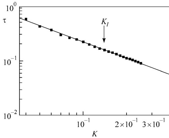
**Fig. 2.** (■) Time lag  $\tau$  between the main Fourier components of interacting chaotic oscillators (11) vs. the coupling parameter  $K$ . The straight line corresponds to the power law  $\tau \sim K^{-1}$ . The arrow indicates the value of coupling parameter  $K_l \approx 0.14$  corresponding to the onset of the lag-synchronization regime.
