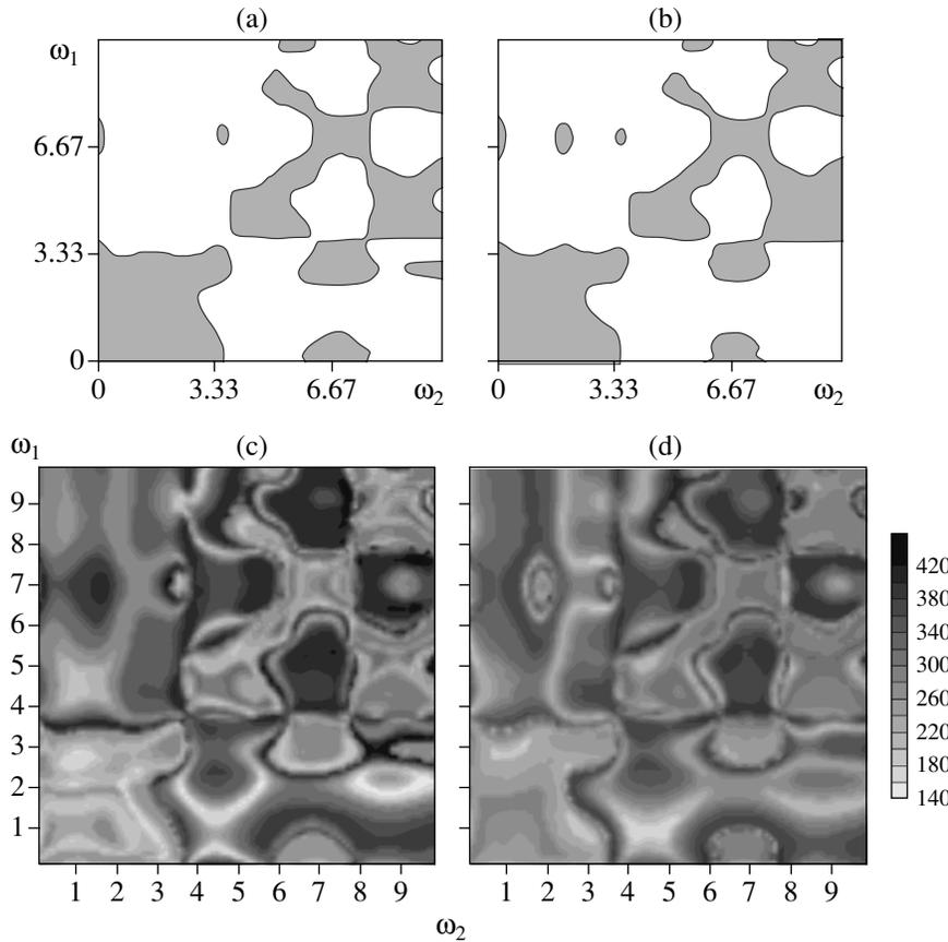
**Fig. 4.** (a, b) Basins of attraction for the slow (white area) and fast (gray area) states and duration of the transient process preceding these states of the CWGS gyro-BWT systems shown on the initial condition plane  $(f_1, f_2)$  (see formula (16)) for  $\alpha =$  (c) 0.8 and (d) 1.0.
