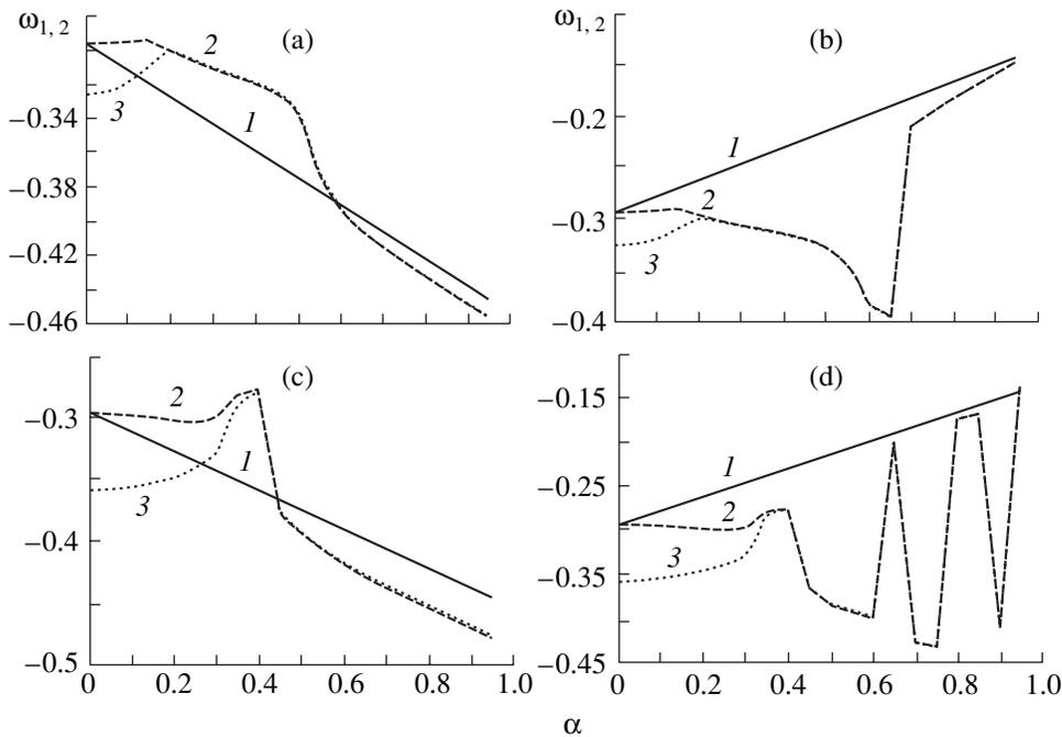
**Fig. 3.** Frequency generated by each of the CWGS gyro-BWTs vs. the coupling coefficient determined at the system lengths  $A =$  (a, b) 3.0 and (c, d) 4.0 for the (a, c) fast and slow (b, d) states of the system: (1)  $\mu_1 = \mu_2 = 2.0$ , (2)  $\mu_1 = 2.0$ , and (3)  $\mu_2 = 3.0$ .
