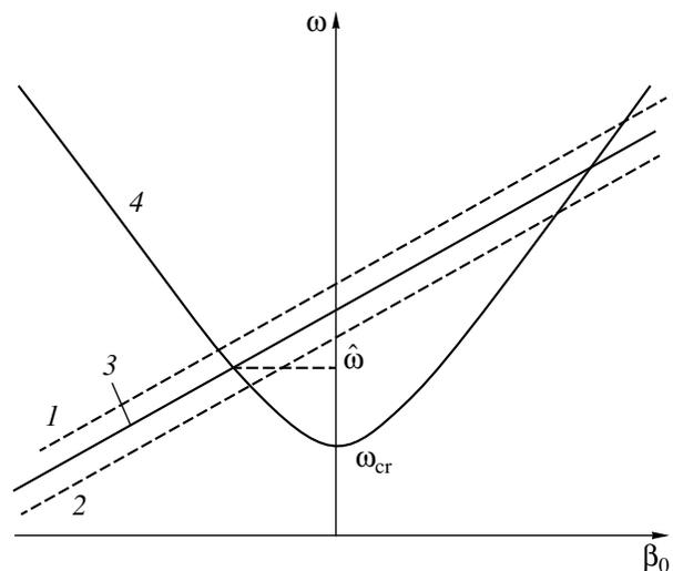
**Fig. 1.** Beam and waveguide mode dispersion curves for oscillations realized in a backward-wave CRM: curves corresponding to the (1) slow  $I_s$  and (2) fast  $I_f$  electron waves, (3) spiral beam, and (4) waveguide mode dispersion curve determined by the formula  $\omega = \sqrt{\omega_{cr}^2 + \beta_0^2 c^2}$ .
