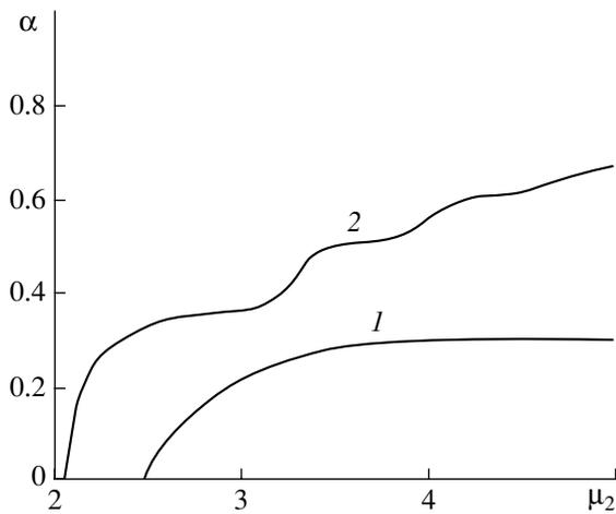
**Fig. 5.** Region of synchronization of joint oscillations of CWGS gyro-BWTs on the nonisochronism parameter  $\mu_2$ —coupling coefficient  $\alpha$  plane obtained at  $\mu_1 = 2.0$ ;  $A = (1) 3$  and  $(2) 4$ .
