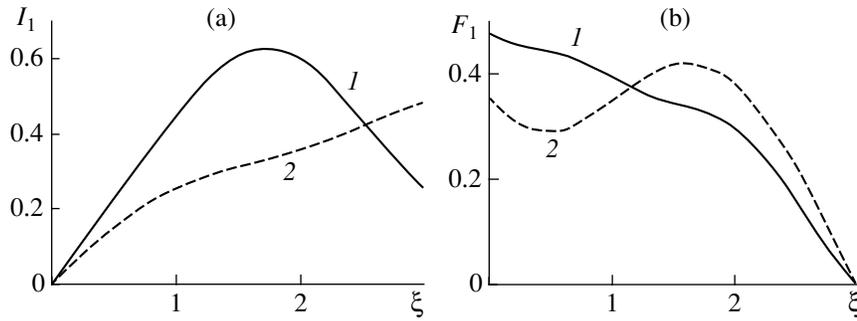
**Fig. 2.** Stationary distributions of RF current  $I_1$  and field  $F_1$  at  $A = 3.0$ ,  $\mu_1 = 2.0$ ,  $\mu_2 = 3.0$ , and  $\alpha = 0.8$  obtained under initial conditions (a) (14) and (b) (15); (1) fast state and (2) slow state. The initial perturbation amplitude is  $\delta^0 = 0.01$ .
