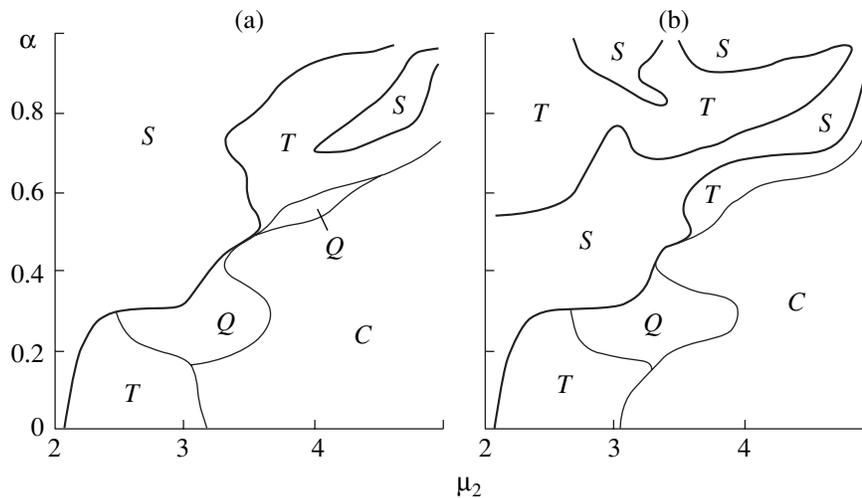
**Fig. 6.** Regions of stationary oscillation and output signal automodulation for the CWGS gyro-BWT joint oscillations on the nonisochronism parameter  $\mu_2$ —coupling coefficient  $\alpha$  plane obtained at  $\mu_1 = 2.0$  for the (a) fast and (b) slow states at  $A = 4.0$ : (area  $S$ ) stationary oscillation, ( $T$ ) periodic automodulation of the output signal, ( $Q$ ) complex periodic automodulation, and ( $C$ ) chaotic oscillations.
