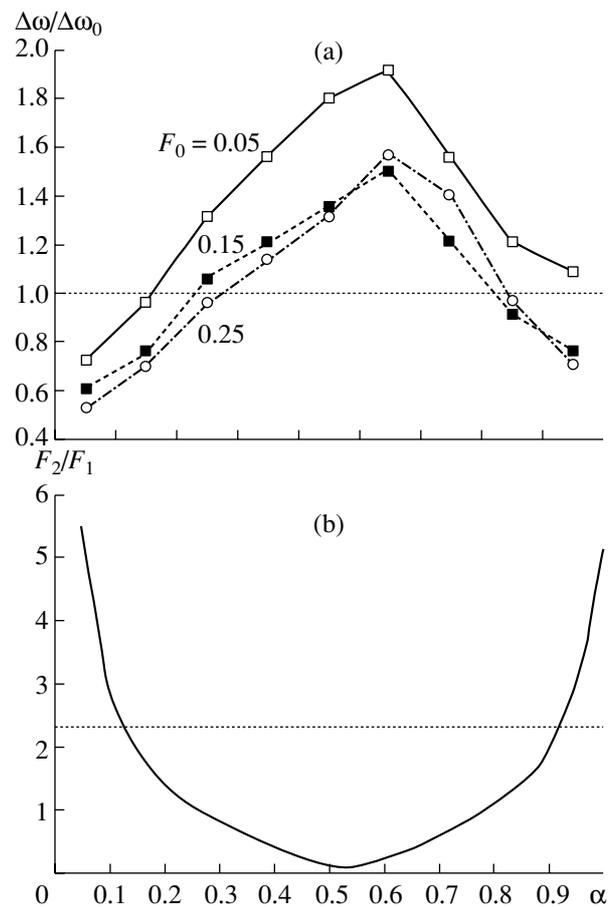
**Fig. 1.** Plots of (a) the normalized synchronization bandwidth  $\Delta\omega/\Delta\omega_0$  for various amplitudes  $F_0$  of the external action and (b) the field amplitude ratio  $F_2/F_1$  at the CWS outputs in the absence of the electron beam versus waveguide coupling coefficient  $\alpha$  for a gyro-BWT–CWS system with distributed introduction of the external high-frequency control signal.
