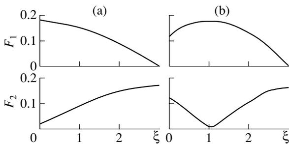
**Fig. 2.** High-frequency field amplitude profiles in the interaction space for “cold” CWSs with  $\alpha = 0.5$  (a) and  $0.8$  (b). The external field with a frequency equal to that of the autonomous gyro-BWT operation is fed to the second waveguide system input ( $\xi = A = 3.0$ ).
