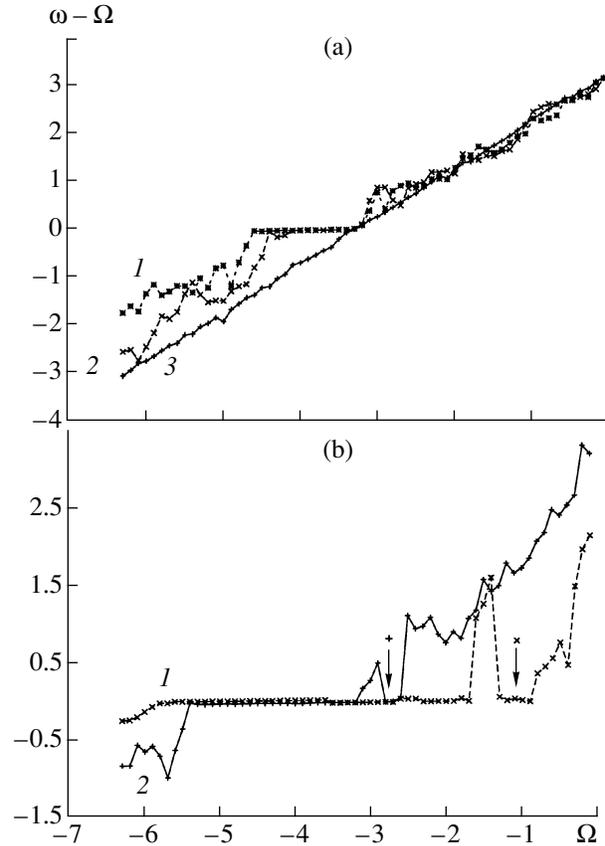
Fig. 3. Frequency difference  $\Omega - \omega$  at the system output as a function of frequency  $\Omega$  at various amplitudes  $F_0$  of the control signal: (a)  $F_0 = (1) 0.22, (2) 0.12,$  and  $(3) 0.02;$  (b)  $F_0 = (1) 0.42$  and  $(2) 0.32$ .
