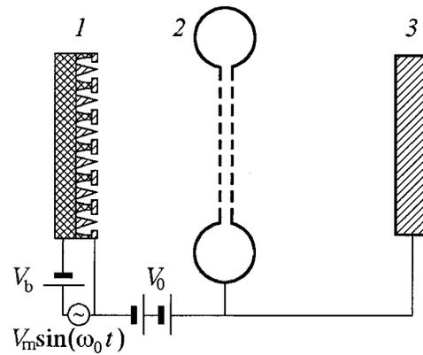
FIG. 3. Schematic of the klystron with FEA: 1—FEA, 2—output cavity, 3—collector.
