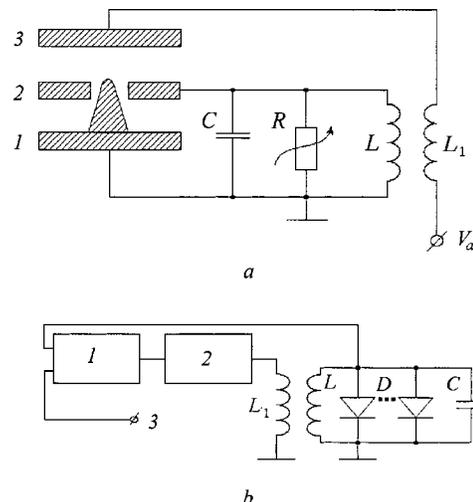
FIG. 8. (a)—Schematic drawing of a self-excited oscillator with field-emission microtriode: 1—emitter; 2—gate; 3—anode; (b)—Circuit analog model: 1—linear amplifier; 2—nonlinear amplifier; 3—external harmonic drive.
