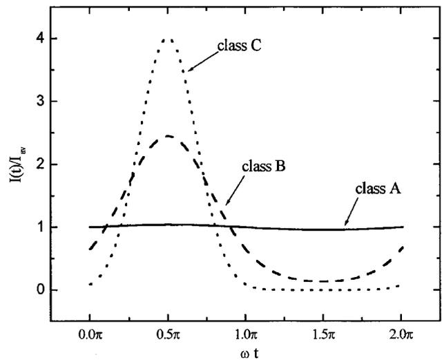
FIG. 10. Current density profile with respect to operation classes.
