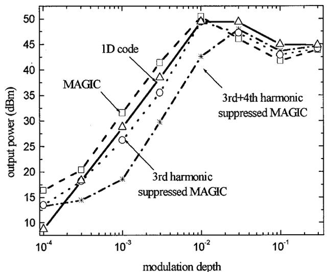
FIG. 11. Output power of twystrode at the saturated position.
