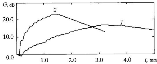
FIG. 6. Gain versus system length for the single-stage (1) and two-stage (2) cross-field amplifiers with FEA.
