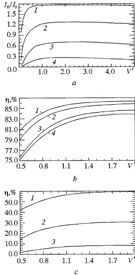
FIG. 4. (a) First four current harmonics  $I_n/I_0$  versus normalized high-frequency voltage  $V'$  calculated according to the Fowler–Nordheim law for  $b' = 10.0$ . (b) Efficiency  $\eta$  of the klystrode amplifier with FEA: 1— $b' = 12.0$ ; 2— $b' = 10.0$ ; 3— $b' = 8.0$ ; 4— $b' = 8.0$ , space-charge effects are taken into account. (c) Efficiency  $\eta$  of the klystrode frequency multiplier for  $b' = 10.0$ : 1— $n = 2$ ; 2— $n = 3$ ; 3— $n = 4$ .
