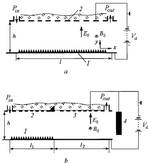
FIG. 5. (a)—Schematic drawing of the single-stage cross-field amplifier with FEA: 1—FEA; 2—slow-wave structure. (b)—Schematic drawing of the two-stage cross-field amplifier with FEA: 1—FEA; 2—input slow-wave structure; 3—output slow-wave structure; 4—collector.
