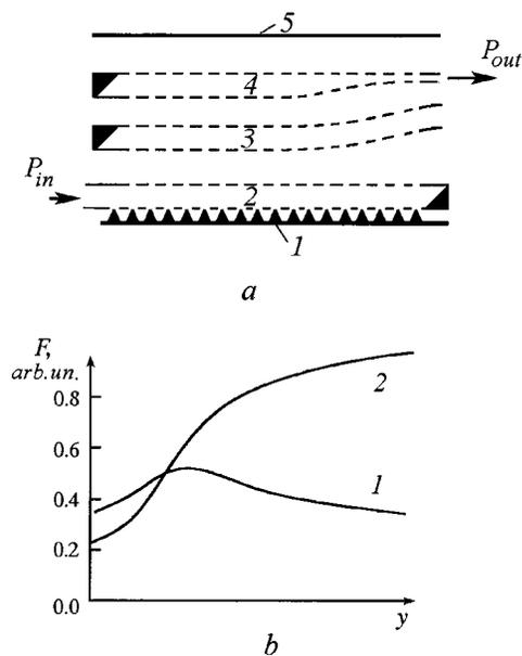
FIG. 2. (a) Schematic of the traveling wave klystron with the intermediate microstrip line (3). Other notations are the same as in Fig. 1(a). (b) Field distributions in the intermediate (1) and output (2) lines.
