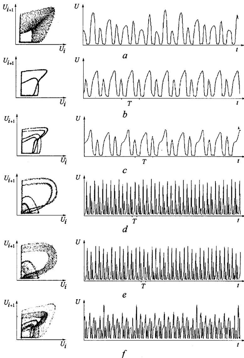
FIG. 9. Experimental voltage wave forms and phase portrait projections for an analog model of the vacuum microtriode oscillator: (a)—quasiperiodic oscillations; (b)—1:2 resonant cycle; (c)—doubled resonant cycle; (d) and (e)—chaotic oscillations; (f)—intermittency.
