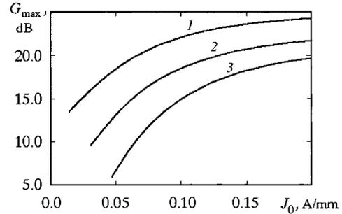
FIG. 7. Maximal gain  $G_{\max}$  versus linear current density  $J_0$  for different values of losses in the slow wave structure for the two-stage CFA: 1— $L = 3$  dB/mm; 2— $L = 6$  dB/mm; 3— $L = 8$  dB/mm.
