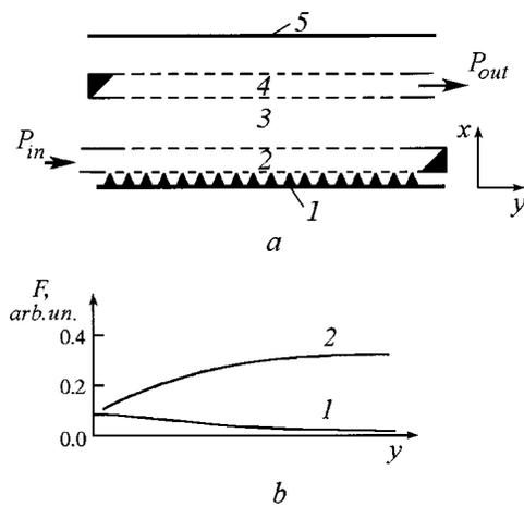
FIG. 1. (a) Schematic of the traveling wave klystron with FEA: 1—FEA, 2—input microstrip line, 3—drift space, 4—output microstrip line, 5—anode. (b) Field distributions in the input (1) and output (2) lines.
